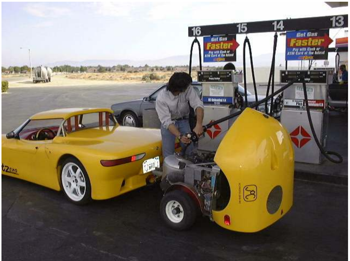
Backtracking genset trailer for "unlimited" range. For AC Propulsion tzero.
