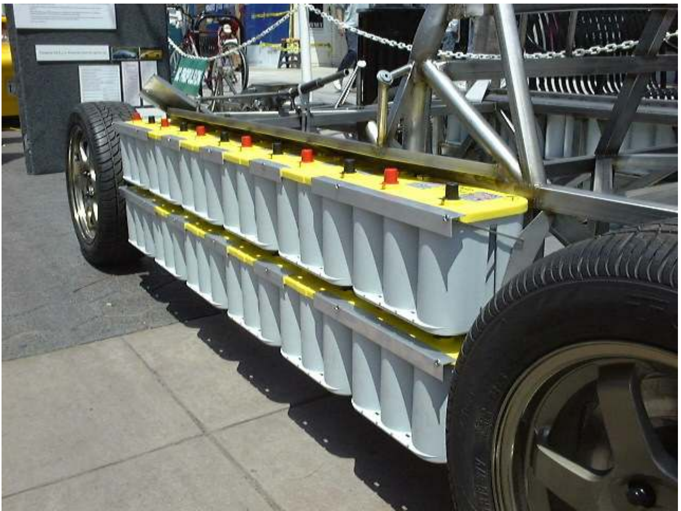
Original lead acid battery pack consisting of 28 Optima Yellow Tops. For AC Propulsion tzero
