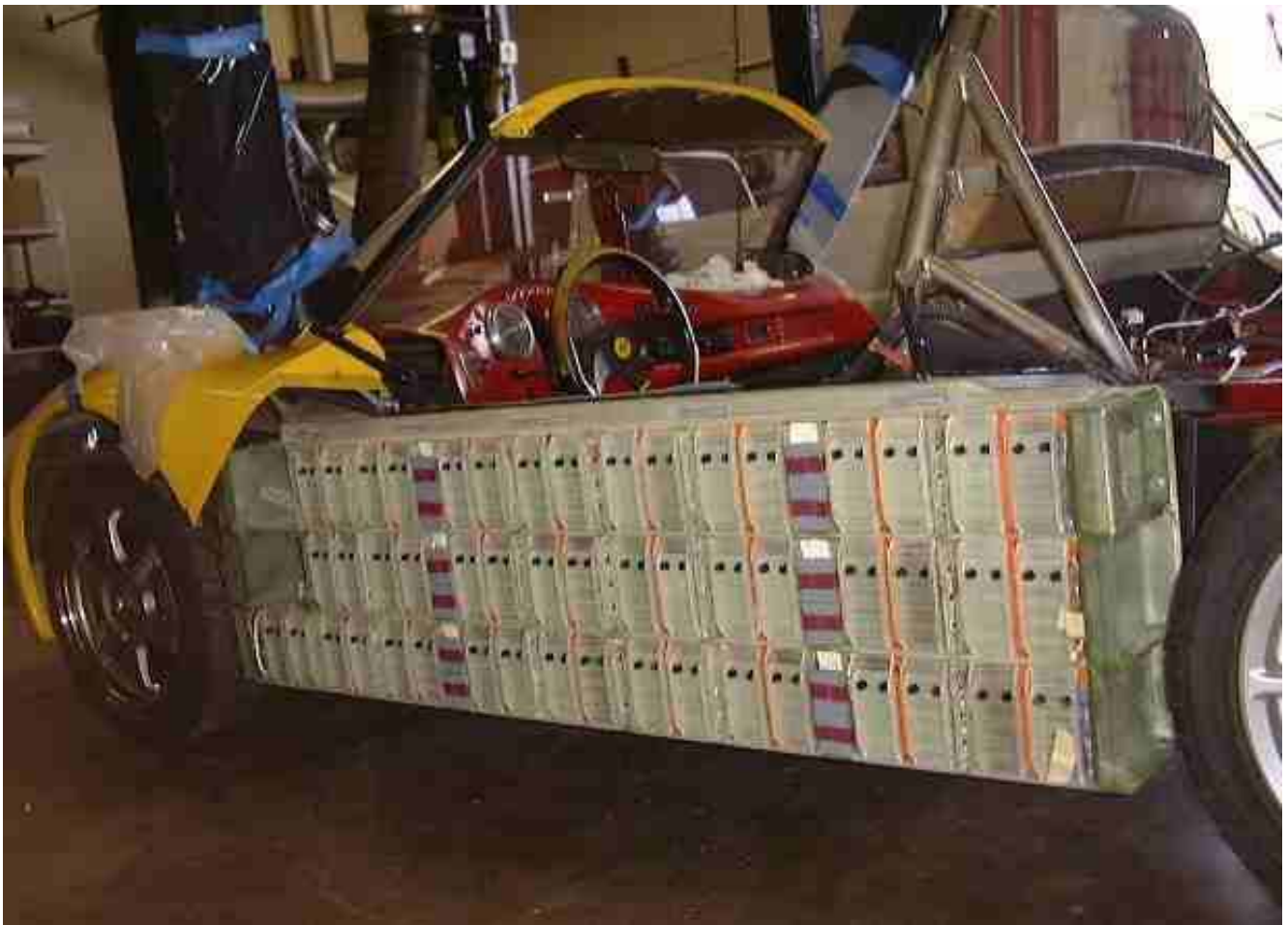
The new Li-ion battery pack for AC Propulsion t 0 . Each of the 100 modules consists of 68 18650 laptop cells.
